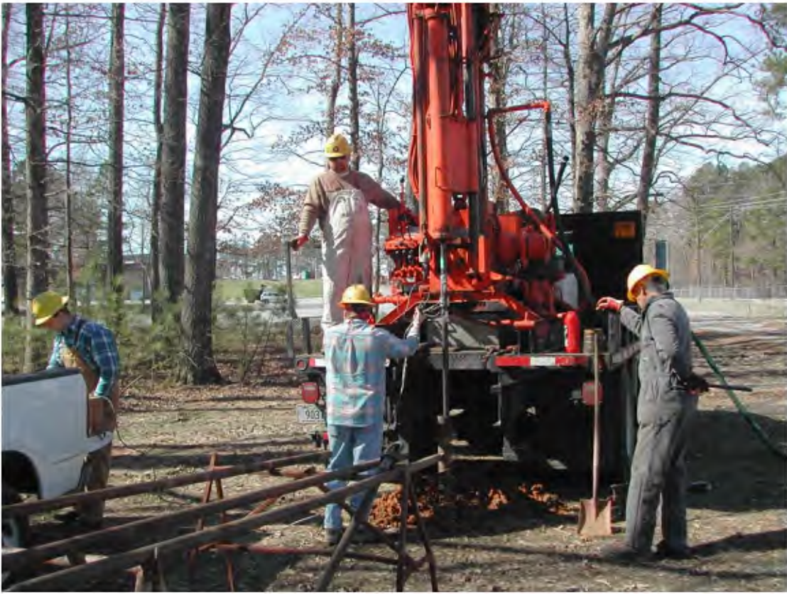
Fig. C-7 CME-45 Skid Rig Testing at Secondary Test Site
